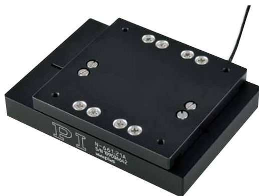
The N-661 miniature linear stage integrates a PiezoWalk® NEXACT® linear motor combined with a high-resolution linear encoder. It provides 20 mm travel and resolution down to the nanometer range.
