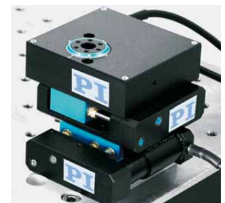
XY \theta_z micropositioning combination consisting of (from top to bottom) M-116 micro rotary stage and two M-111 translation stages (M-110.01 adapter for mounting the M-111 on a honeycomb breadboard with M6 on 25 mm centers)
