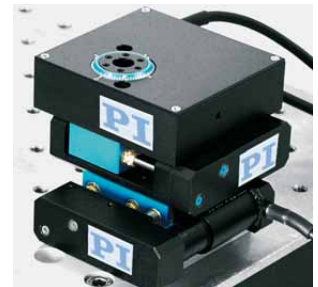
XY \theta_z micropositioning combination consisting of (from top to bottom) M-116 micro rotary stage and two M-111 translation stages (M-110.01 adapter for mounting the M-111 on a honeycomb breadboard with M6 on 25 mm centers)
